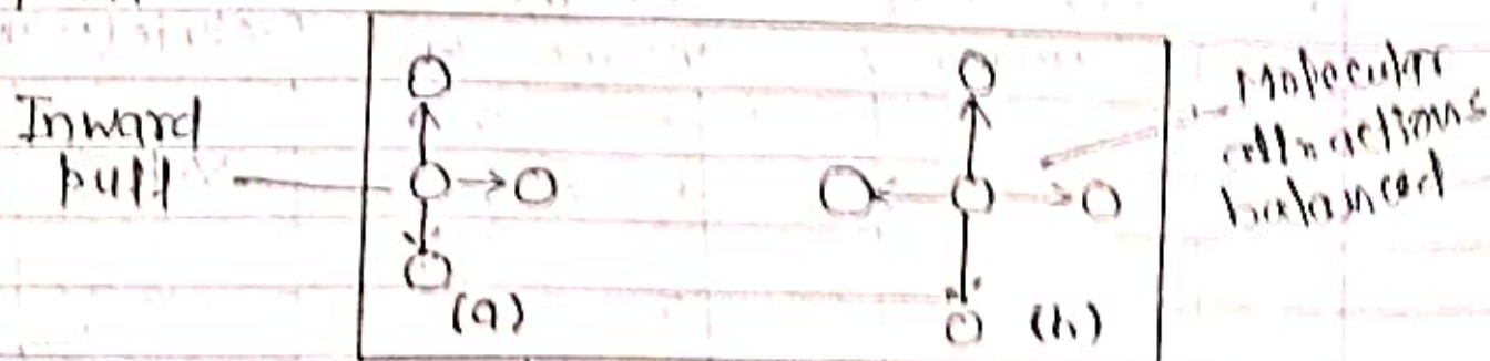
Fig: (a) A molecule about to strike the wall has a net inward pull (b) A molecule in the interior of gas has balanced attractions
